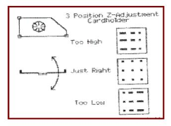
Good system planarity implies that the prober (or device handler for laser trim systems) is checked regularly as part of a routine preventative maintenance program. This will insure that the cardholder and device chuck are flat and parallel to an established reference plane (usually the lead screw axis or air0bearing surface of the prober).
